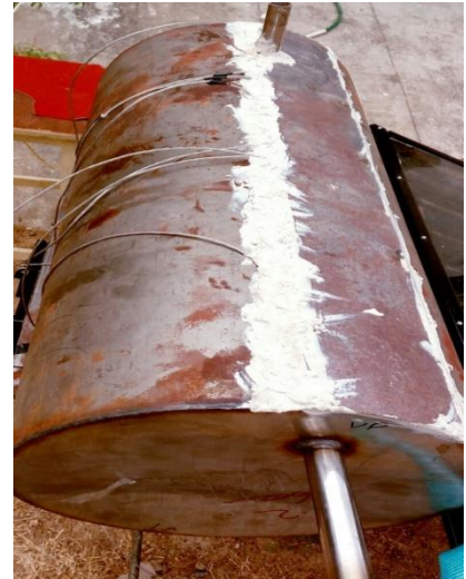
Fig.4 Thermal energy storage (TES) tank
